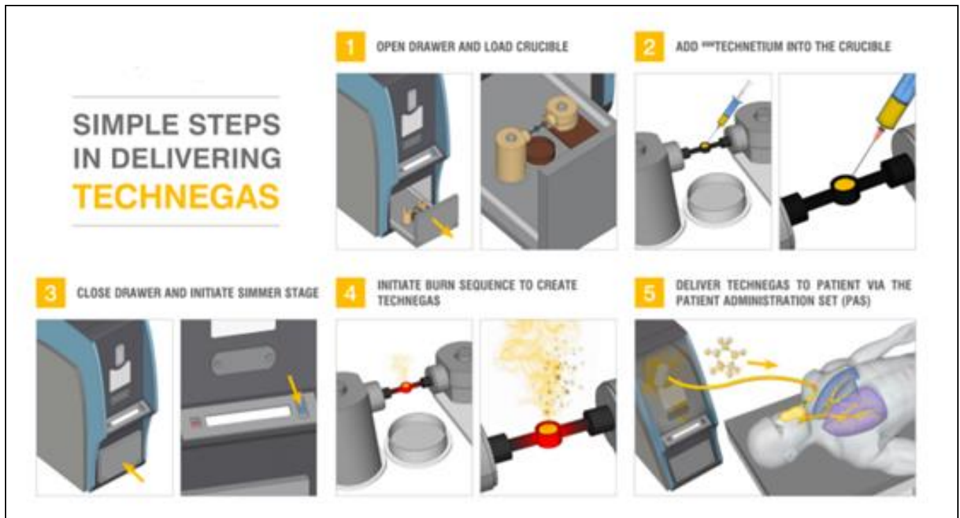
Figure 3: Technegas generation and delivery process
