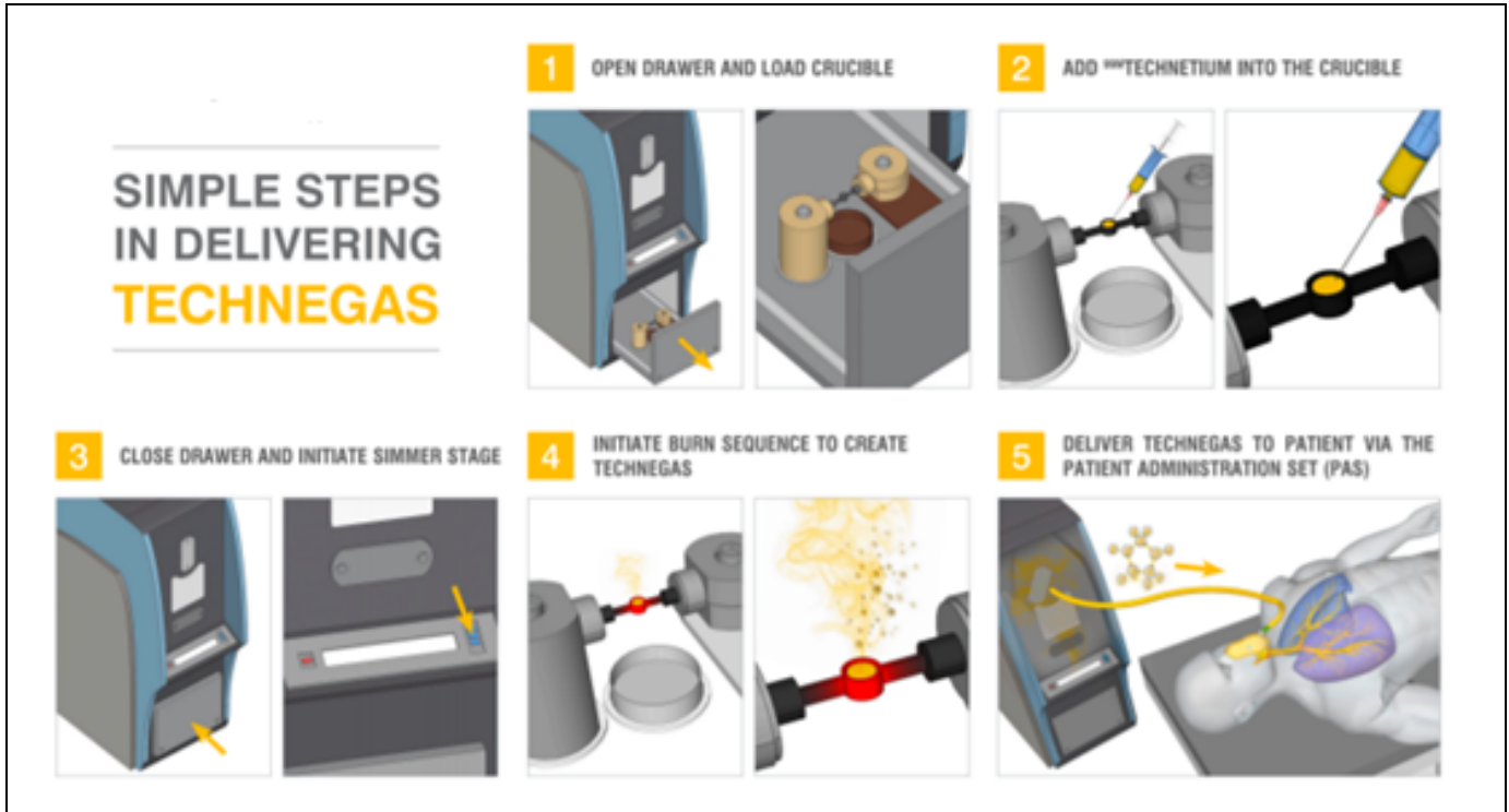
Figure 4: Technegas generation and delivery process
